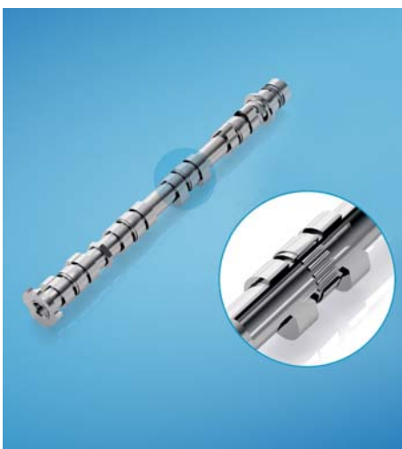
4: Weight-saving construction of a camshaft consisting of a pipe with pressed on, forged cams and integrated single-piece roller bearings. This results in 20 percent less friction loss especially at low rotation speeds (start-stop operation of hybrid drives).
