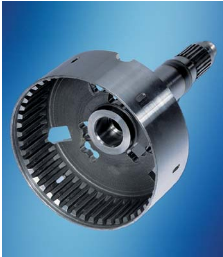
2: Outer disk carriers for the transfer clutch of all-wheel drive vehicles with reduced machining efforts. The basic components is initially produced by means of warm forming. The toothed wheel works are then produced in a cold forming process.
